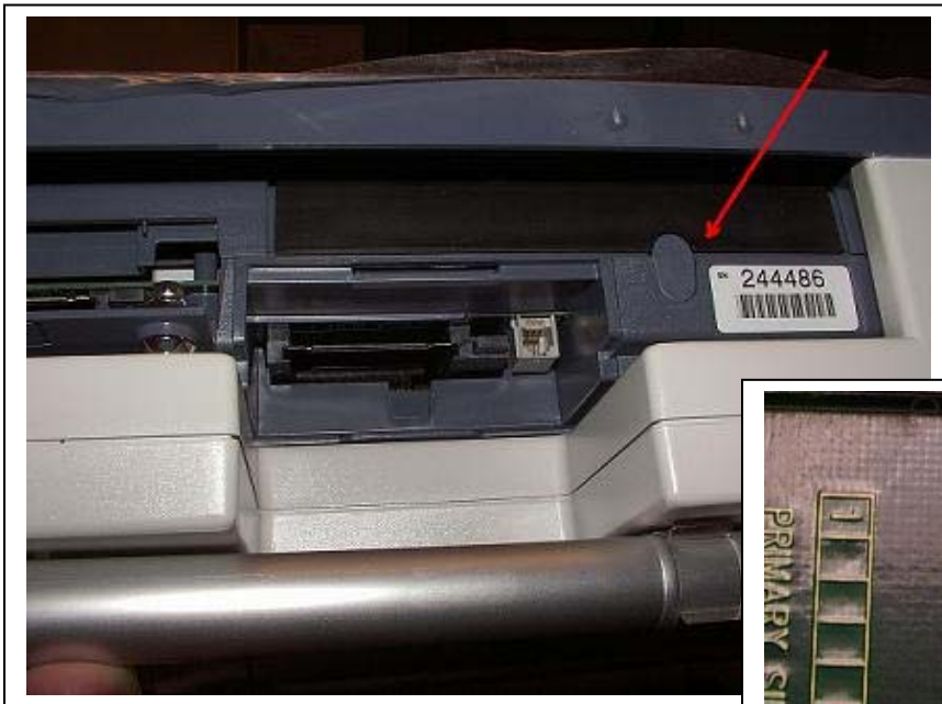
Fig. 6 – Voter-accessible hidden button – Exterior view
